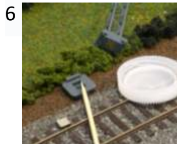
Apply glue to the hole in the base; only in the hole not on the top face of the base
