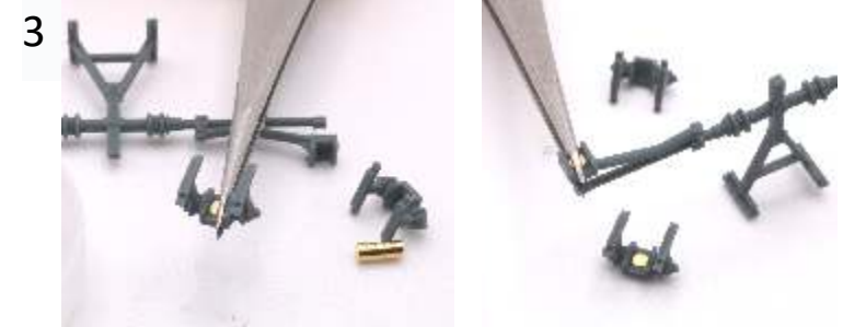
3 Carefully align the magnet with the cup and gently squeeze into place until the magnet is fully home
