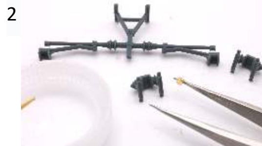
2 Use fine pointed metal tweezers to hold the magnet. Use a cocktail stick to apply a very small spot of glue into the cup in the Registration Arm or Catenary Wire Support
